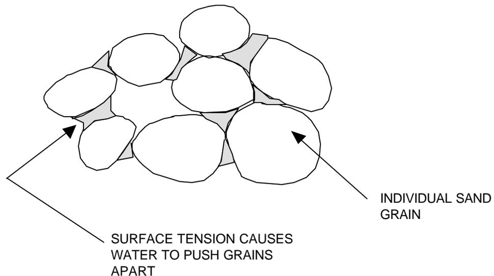
A very dry sand in the hand can not be squeezed into shape whereas a semi moist sand when squeezed could hold some shape until it dries out and crumbles. Surprisingly, addition of more water to saturate the sand collapses the sand as in the very dry state.
