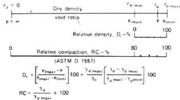
**Figure 8.9** Relative compaction–relative density relationships. (After Lee and Singh, *9th Annual Engineering Geology and Soils Engineering Symposium, Boise, Idaho, 1971.*)
