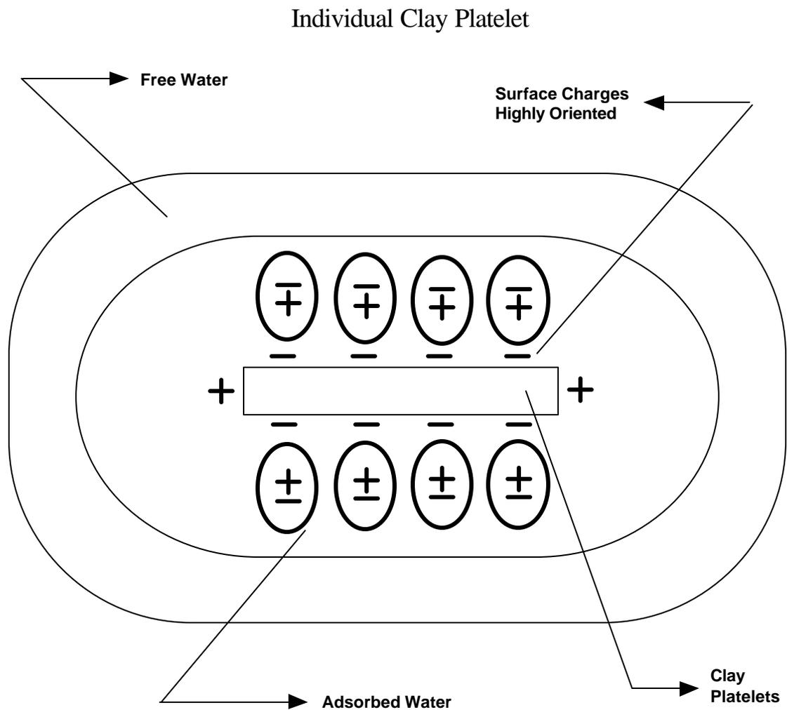
As we can see, the clay is composed of submicroscopic platelets surrounded by Electrical charges, a closely held layer of adsorbed water and an outer layer of
