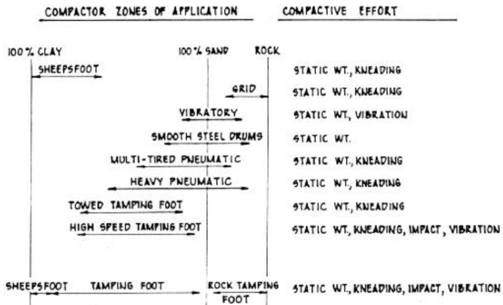
**Figure 8.10** Compaction equipment selection guide. This chart contains a range of material mixtures from 100 percent clay to 100 percent sand, plus a rock zone. Each roller type has been positioned in what is considered to be its most effective and economical zone of application. However, it is not uncommon to find them working out of their zones. Exact positioning of the zones can vary with differing material conditions.
